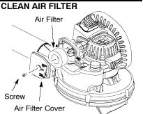
Cleaning the air filter: A dirty air filter decreases engine performance and increases fuel consumption and harmful emissions. Always clean after every 5 hours of operation.
